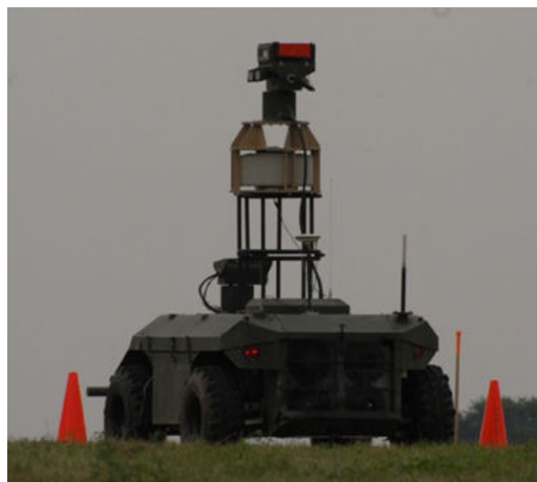
Figure 8: NAUS XUV with mounted IDS radar and LSR pedestal
