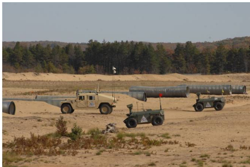
Figure 9: NAUS XUVs in formation following lead HMWVV
